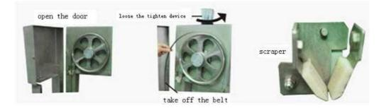
Also it can use the wet slip and hot water and scour to wash the main spare parts ,belt and protective device. Finally, please wipe off all water from the machine by dry cloth.
