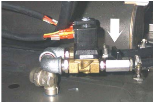
photo 2 Adjustment of flow rate of steam condensate cooling water (optional)
