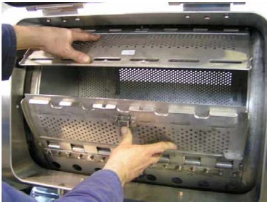
Opening the door, while reducing the hand pressure on the door.
